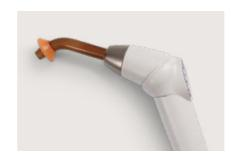
The curing light can be used as a direct version or 120° angled version. With a high-power LED up to a maximum of 2,200mW/cm<sup>2</sup> and a 430 to 490nm emission band, the T-LED lamp offers 6 preset programmes and an optical guide that can be sterilised.
