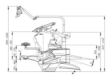
The measures in the drawings are in millimetres.
