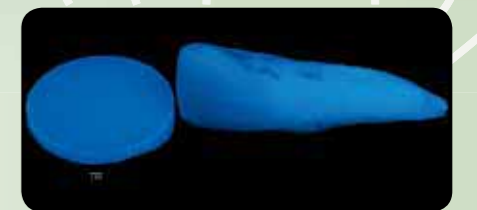
Fluorescence of RelyX™ Ultimate Clicker™ Cement. Source: Courtesy of Dr. Paolo Monteiro
